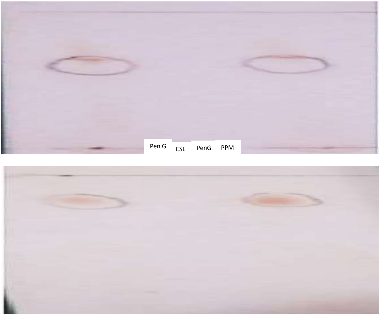
Figuer. (6): TLC technique showed that the crude fungal filtrate extracts appeared spots differed from Rfs of the spots which produced from pure penicillin G.
